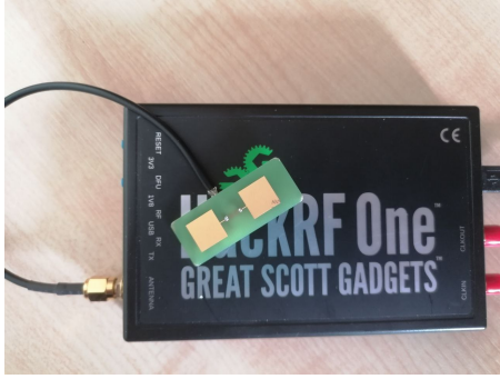
Figure 2: Touch pad with electrodes attached to the SDR.
