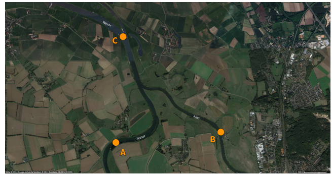
Figure 3: Satellite view of the Aller outfall, DE. The orange dots denote potential measurement stations. Station A is located in the Weser river (left) while station B is located in the Aller river (right), both before the outfall. Station C is located in the Weser river after the outfall. In our example of a trivial model, pollution is detected in C and we aim to assess the likelihood that it could have also been detected in either A or B.
