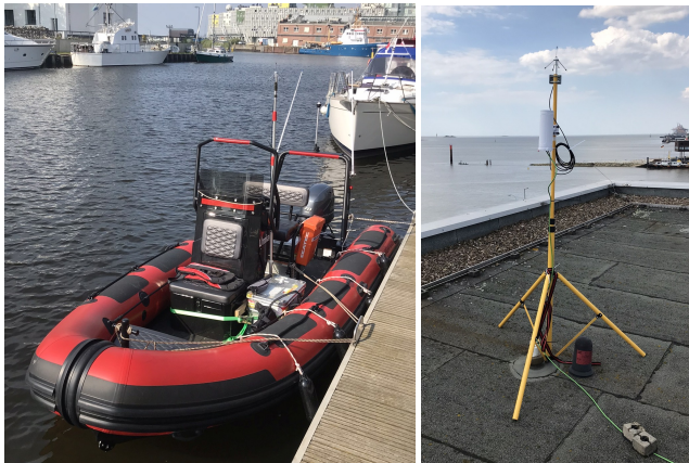
Figure 5: Setup for a range test of the LoRa radio link. Left: motorboat equipped with the sensor node. Right: gateway with a clear view of the river, which serves as the route for the range test.
