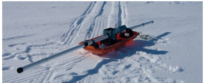
Figure 3: EM31 conductivity meter used to measure sea ice parameters.
