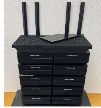
Figure 9: Our testbed: 10 Jetson Nano embedded devices connect to an FL server wirelessly via a TP-Link Router.
