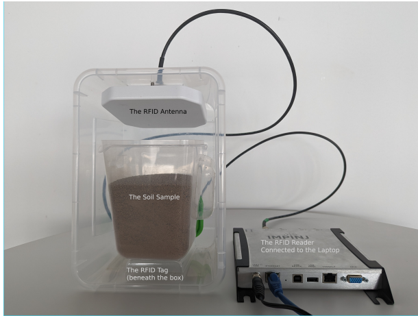
Figure 9: Experiment setup with commercial RFID.
