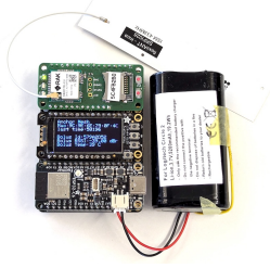
Figure 2: The battery-powered anchor module that contains a LoRa radio with integrated microcontroller (top) and low-power IEEE 802.11 radio with integrated microprocessor (bottom).
